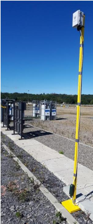
Our solution enables the detection and localisation of any anomalies. The proposed solution offers a capacity of **continuous and real time monitoring** of the entire plant with a capacity to **identify the audio fingerprint of specific events, including fugitive gas leaks**. Using a reliable monitoring system lets the operators focus on the production process.
